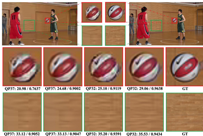
Fig. 2. Artifact level and enhanced result in regions with different frequencies. The second and third rows represent the high-frequency region and the low-frequency region, respectively. The first four columns sequentially represent compressed and enhanced frames under Quantization Parameter QP = 37 , and compressed and enhanced frames under QP = 32 . The raw frame is shown in the last column. PSNR (dB) and SSIM [27] are chosen as objective quality evaluation metric.
