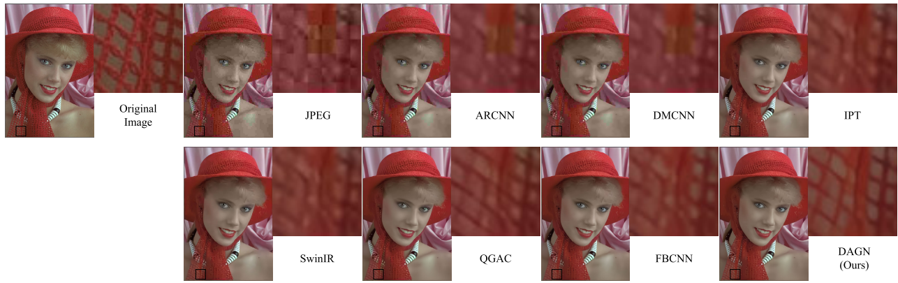
Fig. 9. Qualitative comparisons on Womanhat at QF = 10 . For comparisons, we highlight the regions of interest. Original Image, PSNR | SSIM | PSNR-B. JPEG 27.68 | 0.722 | 26.45. ARCNN [41] 28.36 | 0.753 | 28.34. DMCNN [28] 29.21 | 0.777 | 29.16. IPT [45] 29.36 | 0.778 | 29.32. SwinIR [46] 29.47 | 0.780 | 29.42. QGAC [61] 29.78 | 0.791 | 29.76. FBCNN [13] 29.76 | 0.786 | 29.74. DAGN (ours) 30.03 | 0.793 | 30.03.
