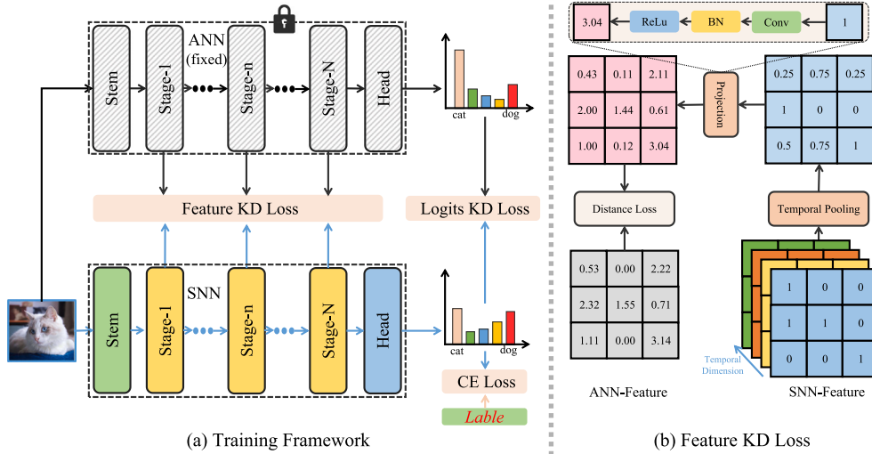
Fig. 3. An illustration of the proposed method, i.e., the knowledge distillations for SNNs. We forced SNNs to learn the feature and logit distribution of pre-trained ANNs with the same architecture. As SNNs and ANNs features are in discrete and continuous space, we use a projection module to map SNNs features to continuous space, matching ANNs features.
