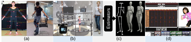
Fig. 4: Human motion data collection methods. (a) Examples of marker-based motion capture setup where (left) optical markers [65] or (right) IMUs [66] are attached to the subject’s body surface. (b) Example of the markerless multiview motion capture system [41]. (c) Pseudo-labeling pipeline involves using pose or mesh estimators to generate pseudo labels [67]. (d) Example interface for manual collection using MikuMikuDance (MMD) resources.
