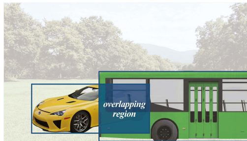
Figure 1: An illustration of the overlapping region. The overlapping region of an object is the tightest bounding box that covers all intersecting areas of its amodal bounding box and those of other objects, so the occluded portion of each object should be inside if exists.
