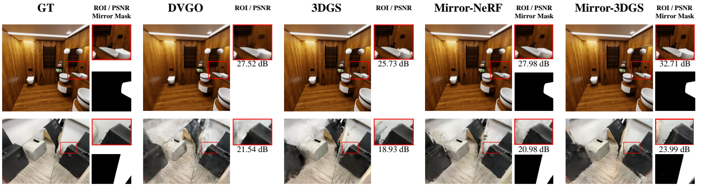
Fig. 4. Qualitative comparison of novel view synthesis. Two rows display washroom and discussion room scenes. The top-right shows magnified mirror regions, and the bottom-right shows predicted mirror masks. PSNR is calculated only for the mirror regions. Both Mirror-NeRF and Mirror-3DGS accurately predict mirror masks, with Mirror-3DGS achieving the best performance.
