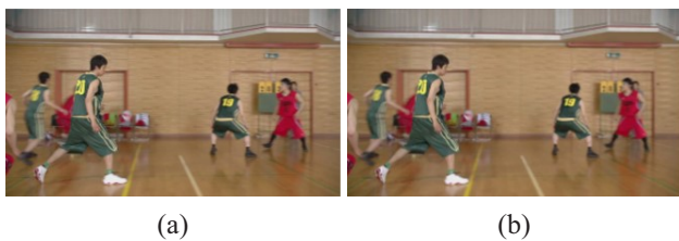
Fig. 5. Subjective comparisons for sequence “BasketballDrive” (a) RD17.0: 29640bits, SSIM: 0.8992, MOS:2.75, (b) Proposed: 19312bits, SSIM:0.8928, MOS:2.67.
