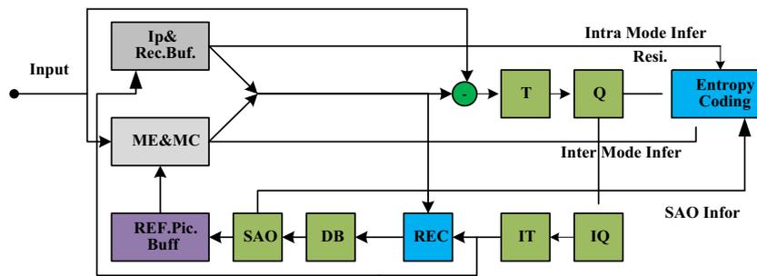
Fig. 2. HEVC hybrid coding framework, IP: Intra prediction, T: Transform, Q: Quantization, IT: Inverse Transform, IQ: Inverse Quantization, REC: Reconstruction, DB: Deblock-filter, ME: Motion Estimation, MC: Motion Compensation.
