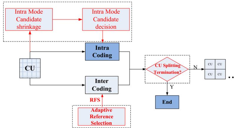
Fig. 1. The architecture of our proposed low complexity RDO scheme.
