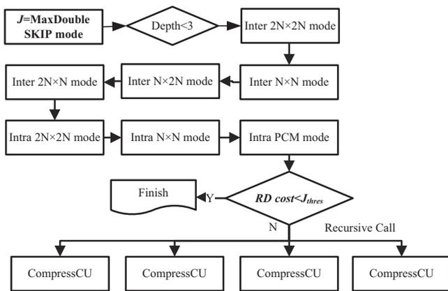
Fig. 8. Architecture of the proposed early termination of CU splitting scheme.
