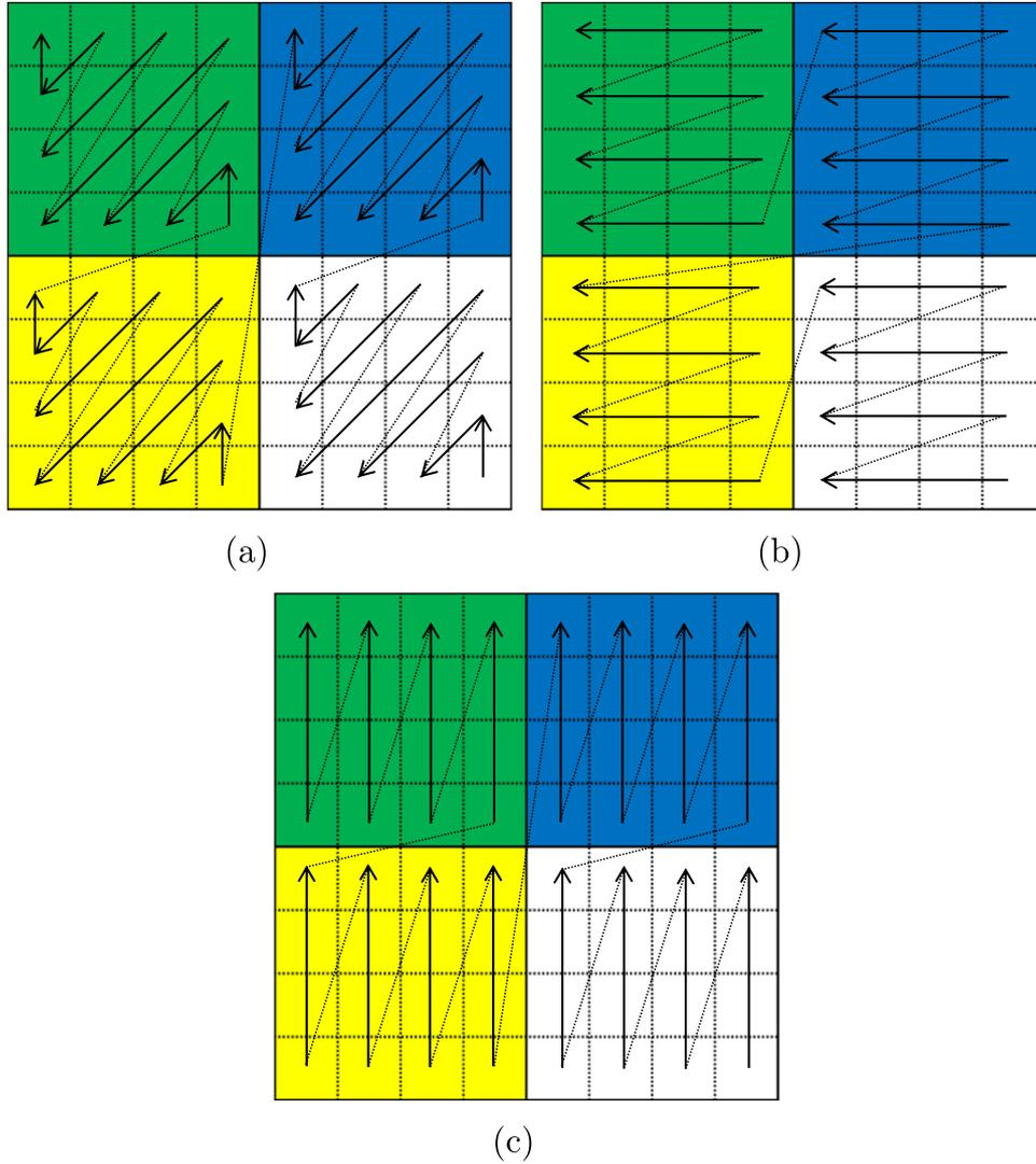
Fig. 1. Sub-block (SB) partition within  $8 \times 8$  TB: (a) diagonal, (b) horizontal, (c) vertical.
