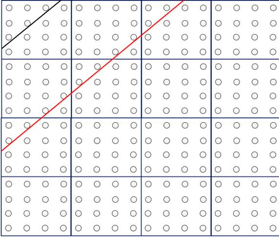
Fig. 7. Splitting method of TBs in luma for coding *coeff\_abs\_greater1\_flag*.
