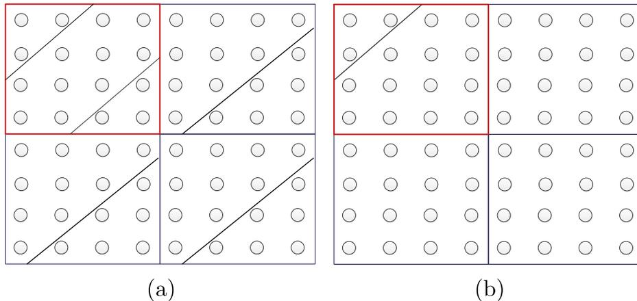
**Fig. 6.** Splitting method of TBs in (a) luma and (b) chroma components for coding *significant\_coeff\_flag*.
