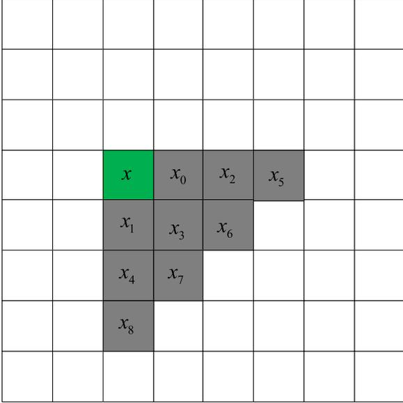
**Fig. 5.** Illustration of the different local templates for the current transform coefficient level  $x$  evaluated in Table 1.
