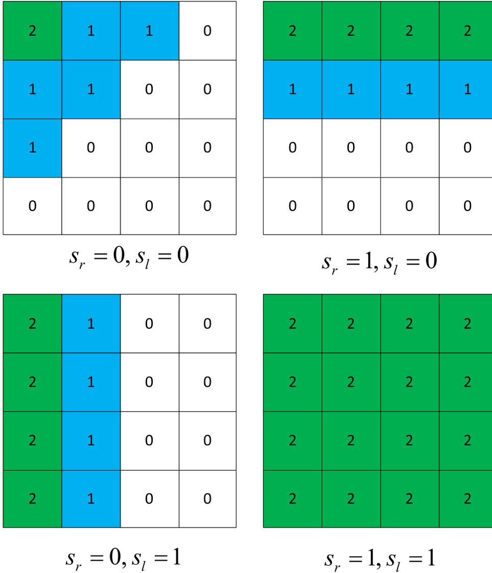
Fig. 3. Templates for *significant\_coeff\_flag* in TBs larger than  $4 \times 4$ .
